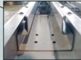
Double "S" shape cross section design
